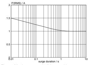
Fig.5. Maximum permissible repetitive rms on-state current  $I_{T(RMS)}$ , versus surge duration, for sinusoidal currents, f = 50 Hz;  $T_{sp} \le 112 \,^{\circ}\text{C}$ .
