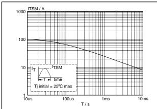
Fig.2. Maximum permissible non-repetitive peak on-state current  $l_{TSM}$ , versus pulse width  $t_p$ , for sinusoidal currents,  $t_p \le 10$ ms.
