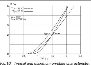
Fig.10. Typical and maximum on-state characteristic.
