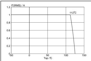
Fig.3. Maximum permissible rms current  $I_{\text{T(RMS)}}$ , versus solder point temperature  $T_{\text{sp}}$ .
