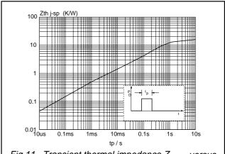
Fig.11. Transient thermal impedance  $Z_{th j-sp}$ , versus pulse width  $t_p$ .
